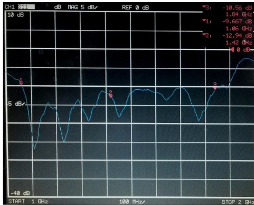
Figure 3.12: Reflection factor  $s_{11}$  as measured by VNA
